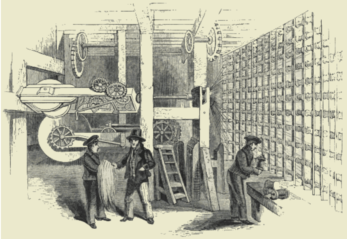
Making Ropes by Huddart's Machinery.
