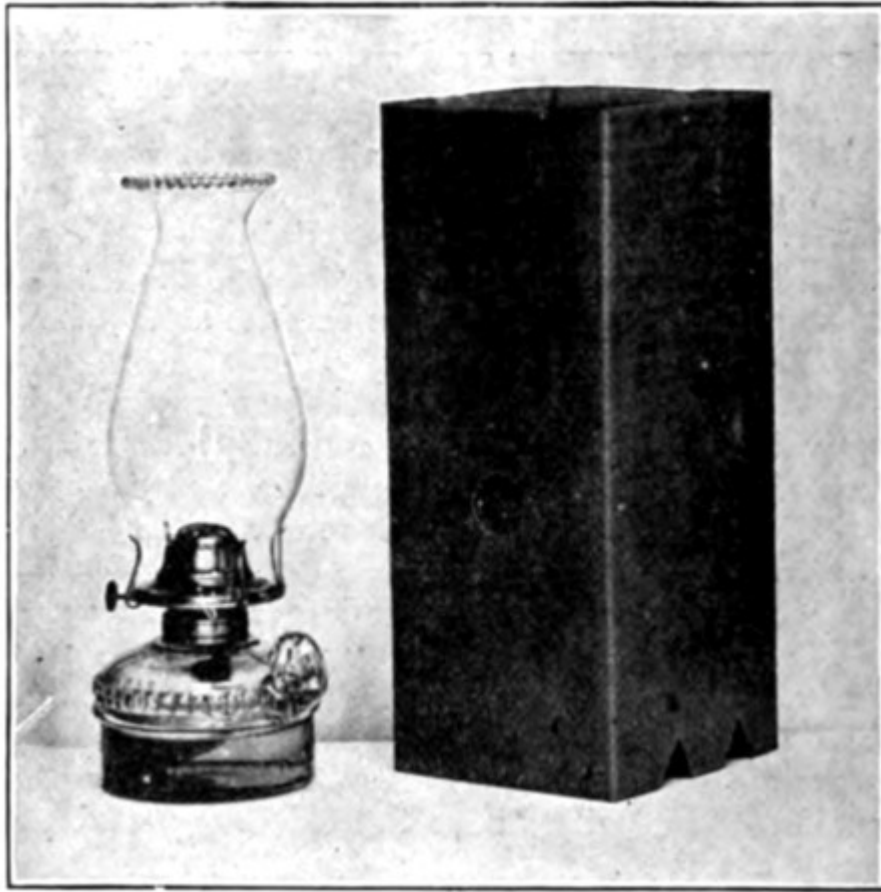
Fig. 1.—This cut illustrates a homemade candling outfit, consisting of small lamp and corrugated pasteboard box.
