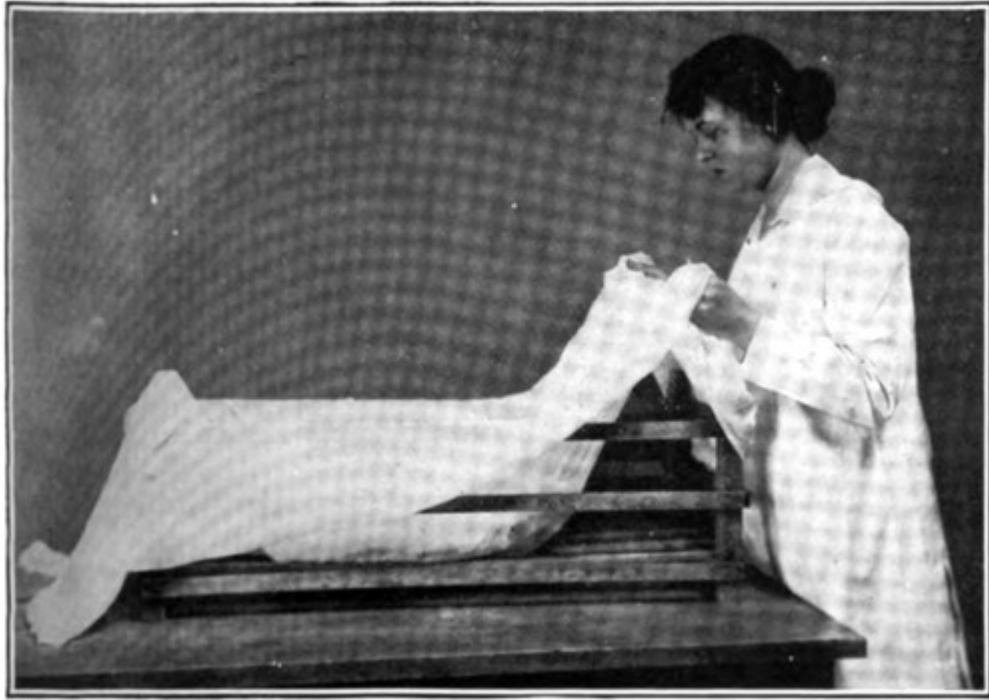
Fig. 4.—Raising and lowering draining cloth to hasten draining.
